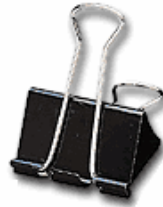
Figure 2: The black portion of the binder clip is tempered spring steel that has been electroplated with a black oxide coating [1]. This material is hypothesized to be 1074 carbon steel [2].
