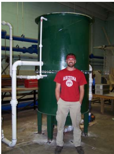
Travis Sorum has fabricated this pressurized constant head tank which will be utilized in his pipe-leak detections project using classical cepstrum method with wavelet filtering.
